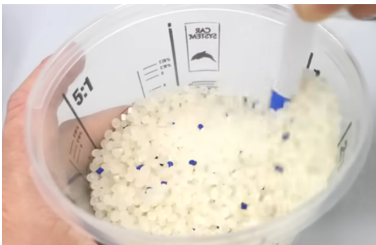
Figure 2 Granular materials with colorant in structure [6]
