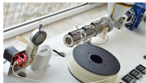
Figure 7 Filament maker from pellet materials [10]
